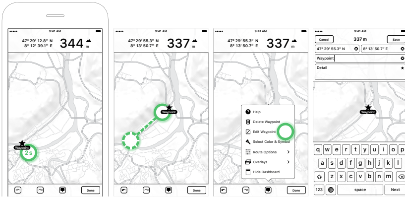
Figure 2.17: Adding a new waypoint by tapping > 2 sec – Move the waypoint by dragging it over the map – Modifying the name or detail of the waypoint – Entering the exact coordinates or title and detail information
