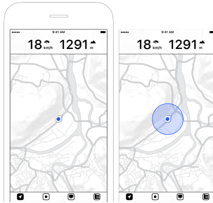
Figure 2.5: Location indicator with heading arrow – Accuracy indicator on location
